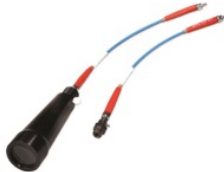
Figure 2. Collimating lenses screw on to the end of SMA 905-terminated optical fibers. The lens at left is best for applications that require collimation of light at long distances in open air.
