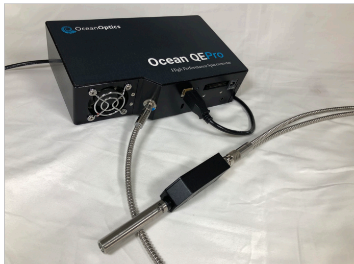
Figure 2. A high-sensitivity spectrometer like the QE Pro-Raman+ can be combined with the appropriate laser and probe for convenient Raman analysis of a wide range of samples.
