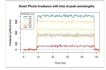
While the spectral stability of the flash appeared quite high, we were curious to look at it more closely. A color temperature plot over time showed a slight upward trend in color temperature, roughly 500 K over 15 ms. This was supported by high color consistency as shown in the very stable chromaticity diagram plot. With zooming, we would see on the plot that flash color varied by <0.02 in x and y over the lifetime of the three flashes measured.
