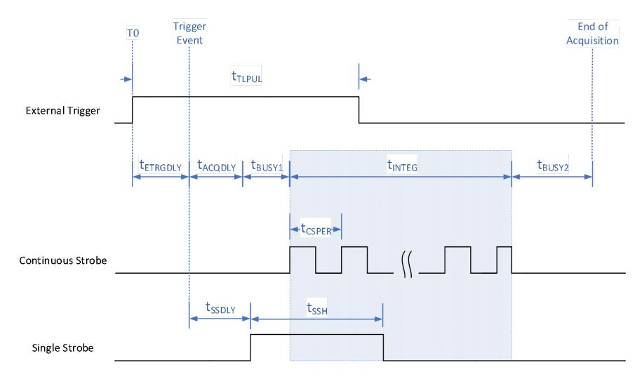
External Level Trigger timing characteristics are defined in the tables below.
