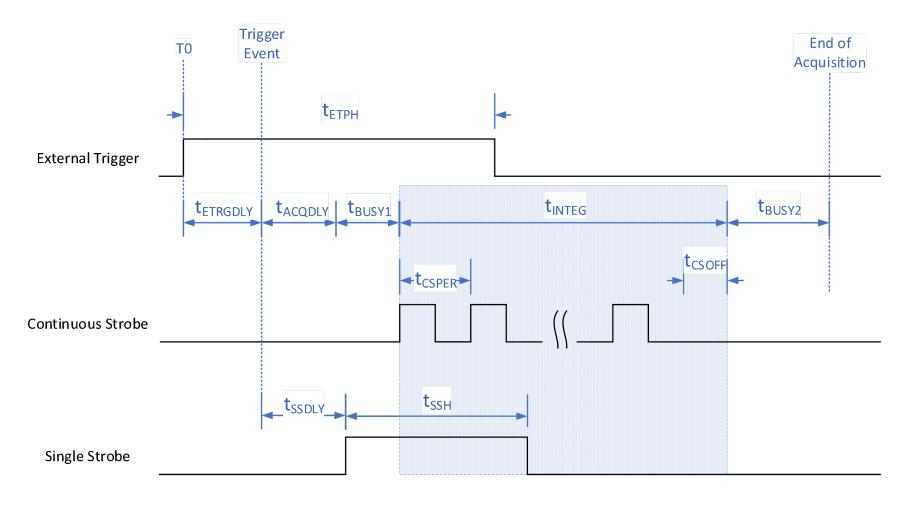
Figure 2 External Edge Trigger Timing Diagram
